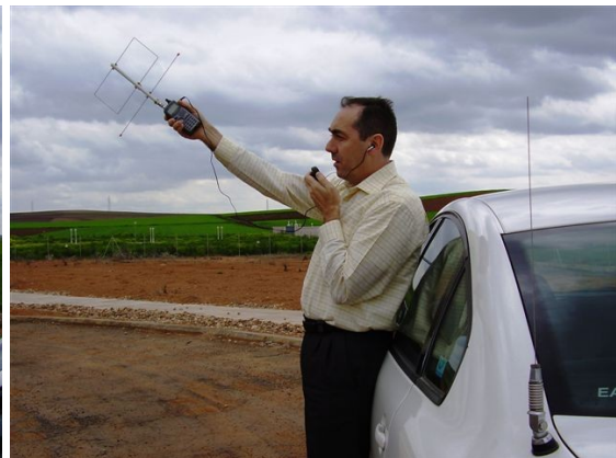
Photo n°6: Complete EA4CYQ mobile/portable station. A 1/4\lambda whip on the car roof to uplink and the ‘CJU’ in the downlink.
