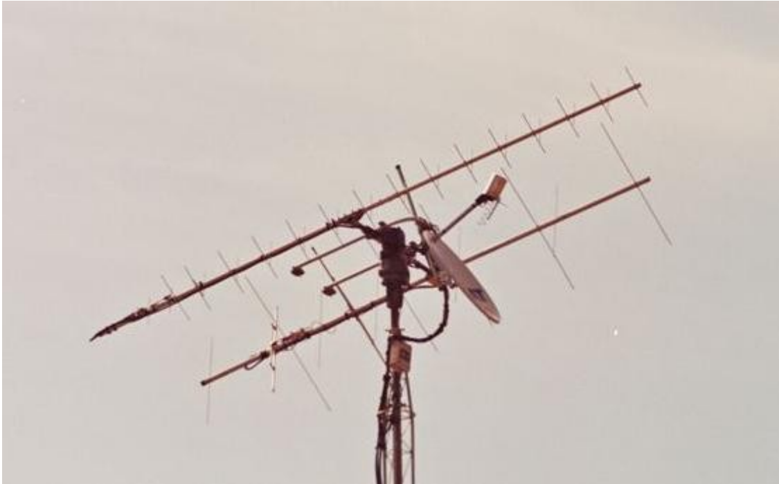
Side view of a typical aerial system of a base station for amateur satellites
