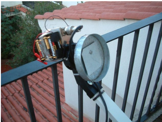
Photo n°6: A ringed patch-feed attached to a downconverted supplied by work in portable of
