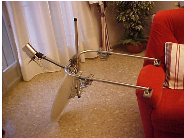
Photo n°9: Detail of the structure to support the dish, you can see the counterweights
