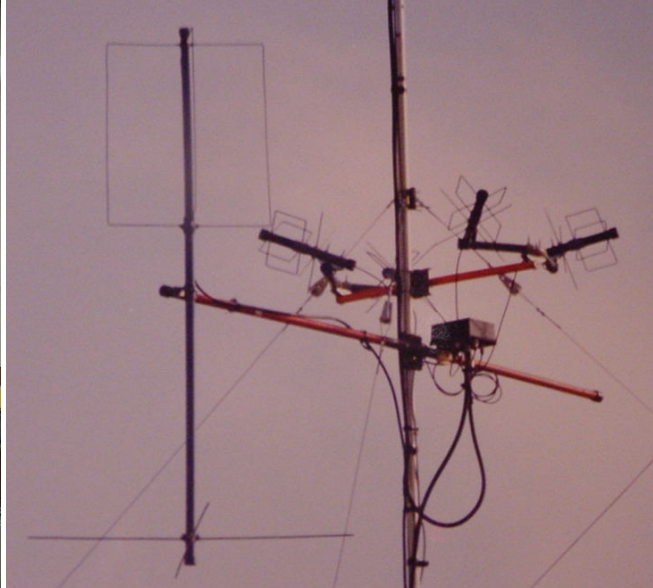
f) Eggbeater of VHF + 4*TPM II of UHF (The roof of my fix station)
